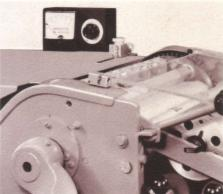
**Ink Monitor . . . (optional equipment)**Accurately and continuously measures amount of ink in inking system. Enables operator to maintain color uniformity.
