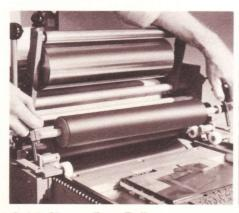
**Quick Change Form Rollers...**Integrated construction of nylon bearings and height adjustment permits rollers to be changed in seconds.
