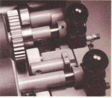
Form Roller Support System . . . Form roller contact is controlled by the press bed bearers for the most exacting requirements.
