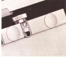
**Sheet Guide Adjustment Knobs..**Micrometer-type, wider knobs for easier turning, more accurate operation.
