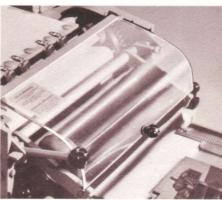
**Curved Plastic Cover...**For protection against inking system contamination.
