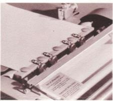
**Foot Operated Gripper Bar...**Provides positive gripping for wide range of sheet sizes.
